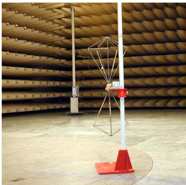
PBA 320 antenna pair for normalised site attenuation testing in a semi anechoic chamber
